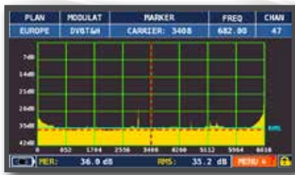
MER vs CARRIER Reverse visualization.
