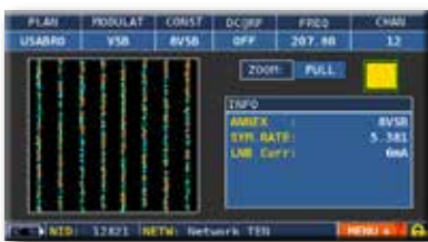
VSB constellation, on the right relative modulation parameters
