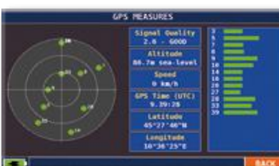
GPS antenna Quality, constellation & Position.
