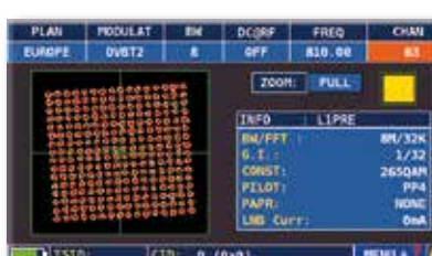
DVB-T2 (opt.) rotated Constellation 256 QAM mod., on the right relative modulation parameters & M-PLP
