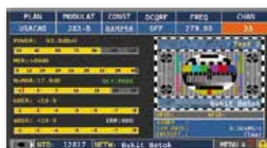
J83-B signal, all the measurements, picture and settings on one screen
