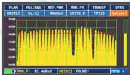
Example pointing Hot Bird 13 ° East The tool informs you that the dish is oriented on the correct satellite via the message HBT13 FOUND!
